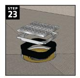
Loosely fit the HYDRO-BLOK stainless steel drain and tray into the shower pan drain opening while installing tile (tile up to the edge of the tray).
