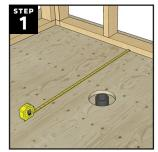
Install the Shower Pan and Drain Kit. Measure the area where the shower pan will be installed to determine if the pan must be cut to size. Pay attention to the drain location when cutting a shower pan to size. We recommend leaving a ¼" space between the pan edge and the framed wall.
