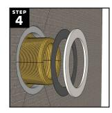
Carefully place the shower pan on edge and slide the rubber gasket and then the fiber gasket over the drain body threads while firmly holding the drain body from the front to ensure it remains seated in the shower pan.
