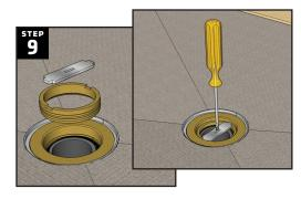
Thread the solid brass caulking nut into the drain body to compress the rubber gasket onto the 2" drain pipe. Once it is hand tight. take the flat tightening key and place it into the solid brass caulking nut and then further tighten with a large flat screwdriver by placing the screwdriver in the slit in the middle of the tightening key.
