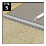
Use masking tape or duct tape to mask off the entire drain opening 1 ½" from the rear edge of the linear drain body to ensure no sealant enters the drain.
