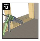
Apply a 1/2" continuous bead of joint sealant in the side shower pan channel and down the edge of the rear wall board so that the side wallboard can be pressed firmly into the shower pan channel and against the rear wallboard.
