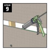
When placing a new piece of wallboard on top of an existing one, apply a  $\frac{1}{2}$ " bead of joint sealant along the entire edge of the lower board. Press the new wallboard firmly into the joint sealant and hold against the studs. Install a washer and screw 12" up from the seam close to the to center of the board to provide initial support.
