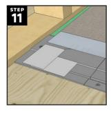
Apply strips of masking/duct tape to cover the end of the HYDRO-BLOK linear drain opening. Ensure at least 1-2" of the drain opening at each end is masked to prevent joint sealant from entering the drain.
