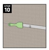
Install washers and screws along the seam before continuing to add washers and screws at 12" intervals to secure the board to the studs.
