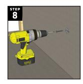
Fasten the wallboard to the studs using HYDRO-BLOK screws and washers Place the first washer 12" up from the bottom of the shower pan and screw it in flush to the surface of the wallboard. Continue placing washers and screws every 12" along each stud until the entire sheet is fastened to each stud.
