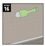
Remove the masking /duct tape mask from the linear drain ends before the joint sealant cures.
