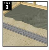
Mark a line on your subfloor 1" from the edge of the linear drain body. Apply modified thinset to the subfloor starting at the back of the shower area, troweling towards the front and stopping at the marked line.
