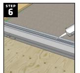
Cut a length of the 2" mesh tape supplied with the shower pan to the length of the seam. Press the mesh tape into the seam, carefully pressing it into the joint sealant.
